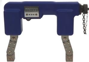
The KDE MP-A2 electromagnetic AC yoke is a low cost, portable instrument which provides fast and accurate defect detection in ferrous metals. The yoke features a dual coil which induces a powerful magnetic field providing maximum lifting power and flux density without uncomfortable heating.
